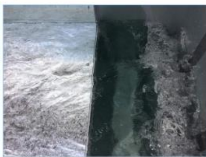
DB 600-1, Q = 16 l/s (box gutter slope - 1 in 200)
