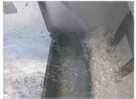
DB 300-1, Q = 16 l/s (box gutter slope - 1 in 200)
