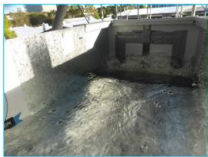
DB 300-1, Q = 16 l/s (box gutter slope - 1 in 200)
