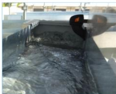
DB 200-1, Q = 16 l/s (box gutter slope - 1 in 200)
