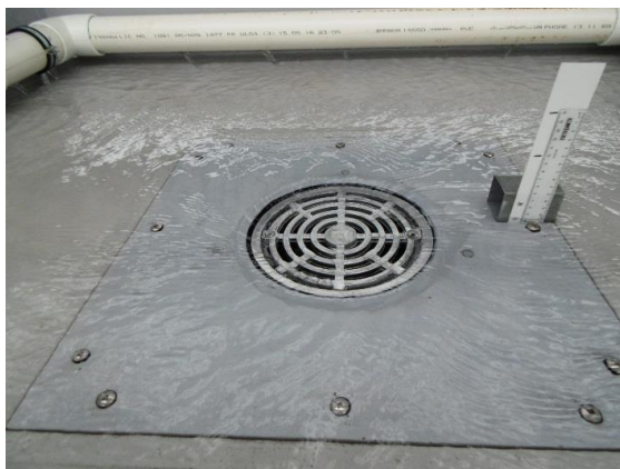
Weir Flow – 3 L/s (13mm)
