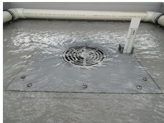
Surcharged flow – 4 L/s (20mm)
