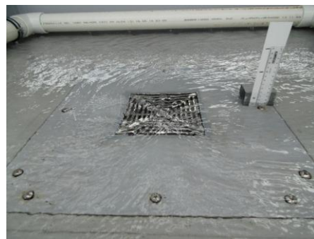
Surcharged Flow 4 L/s (27mm)
