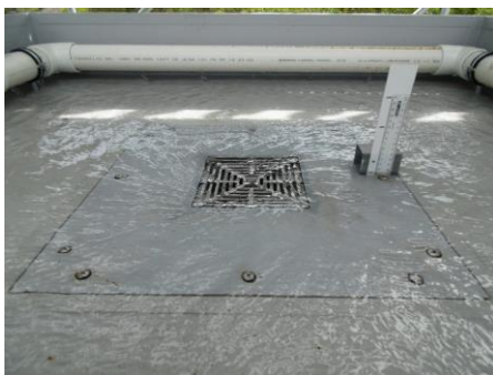
Weir Flow – 2 L/s (20mm)
