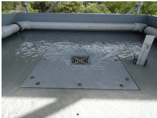
Weir flow - 1 L/s (20mm)
