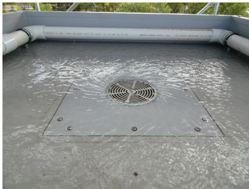
Weir flow - 1 L/s (10mm)
