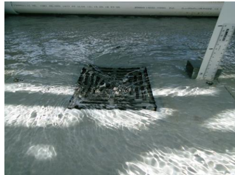
Orifice Flow – 6 L/s (30mm)
