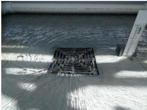
Weir Flow – 4 L/s (25mm)
