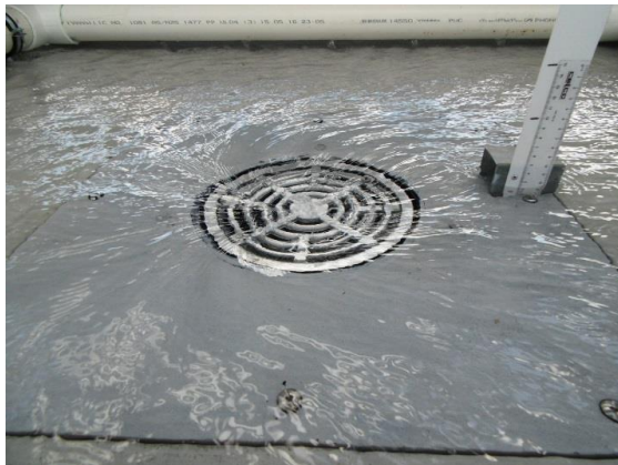
Weir Flow 8 L/s (30mm)
