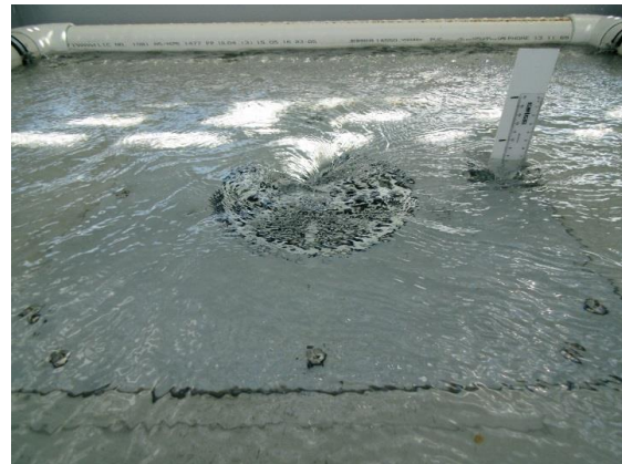
Surcharged flow 12 L/s (90mm)
