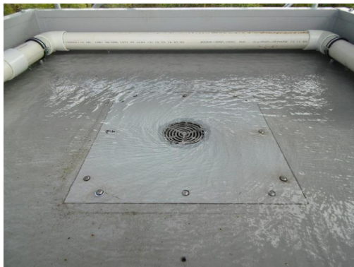
Weir flow - 1 L/s (25mm)
