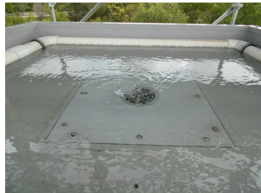
Surcharged flow – 3 L/s (75mm)
