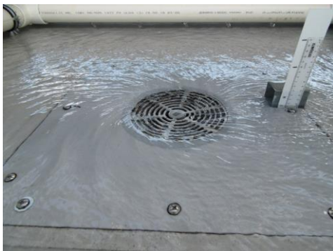
Weir Flow – 2.5 L/s (15mm)
