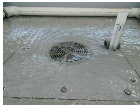
Surcharged flow – 4 L/s (30mm)
