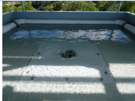
Orifice Flow - 3.0 L/s (80mm)
