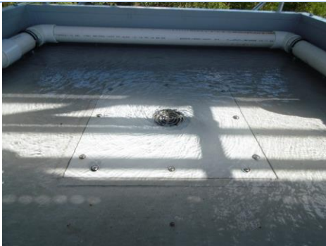
Weir flow - 1 L/s (40mm)
