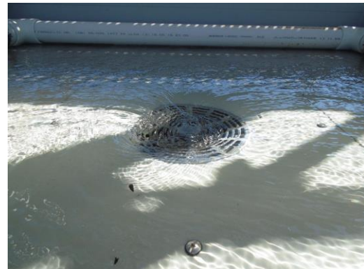
Choked Flow – 6 L/s (42mm)
