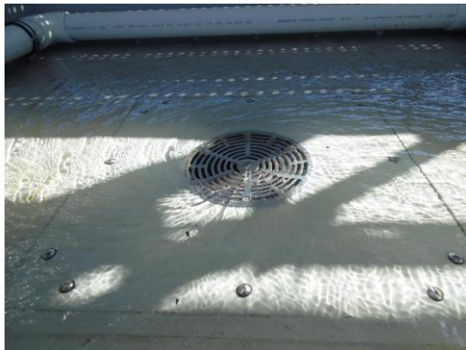
Weir Flow – 2.5 L/s (30mm)
