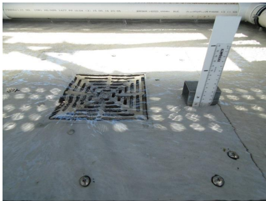
Weir Flow – 6 L/s (18mm)
