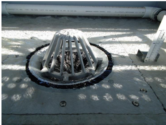
Weir Flow 18 L/s (42mm)
