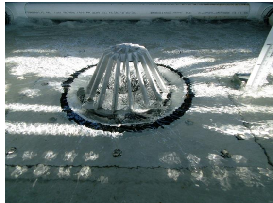
Surcharged Flow - 20 L/s (40mm)
