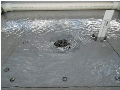
Weir Flow – 2.5 L/s (50mm)
