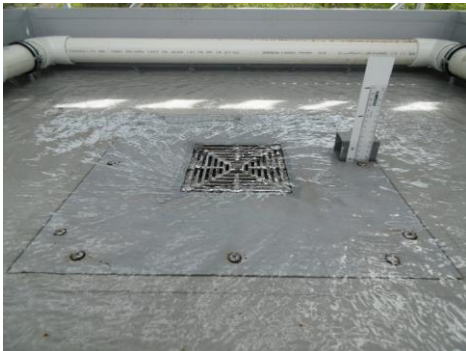
Weir Flow – 2.0 L/s (20mm)
