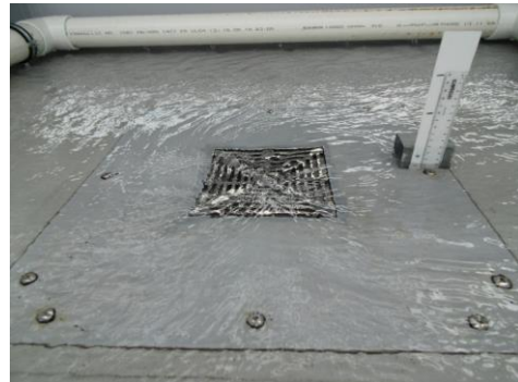
Orifice flow – 4.0 L/s (30mm)
